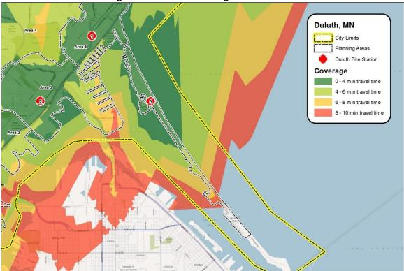
Figure 18: Current Coverage with Station 5
