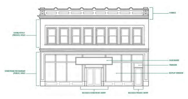
Figure 5: Diagram showing two-part commercial block.
