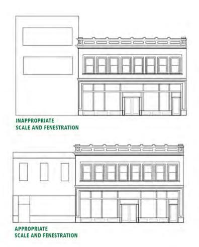
Figure 12: Diagram showing scale and fenestration for new construction and additions.
