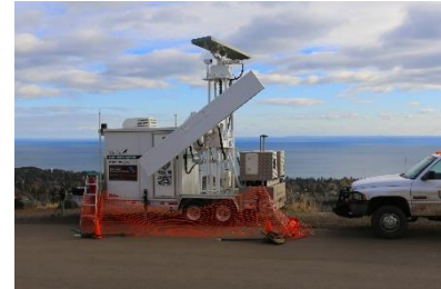
An avian radar system in Hawk Ridge tracking bird activity
