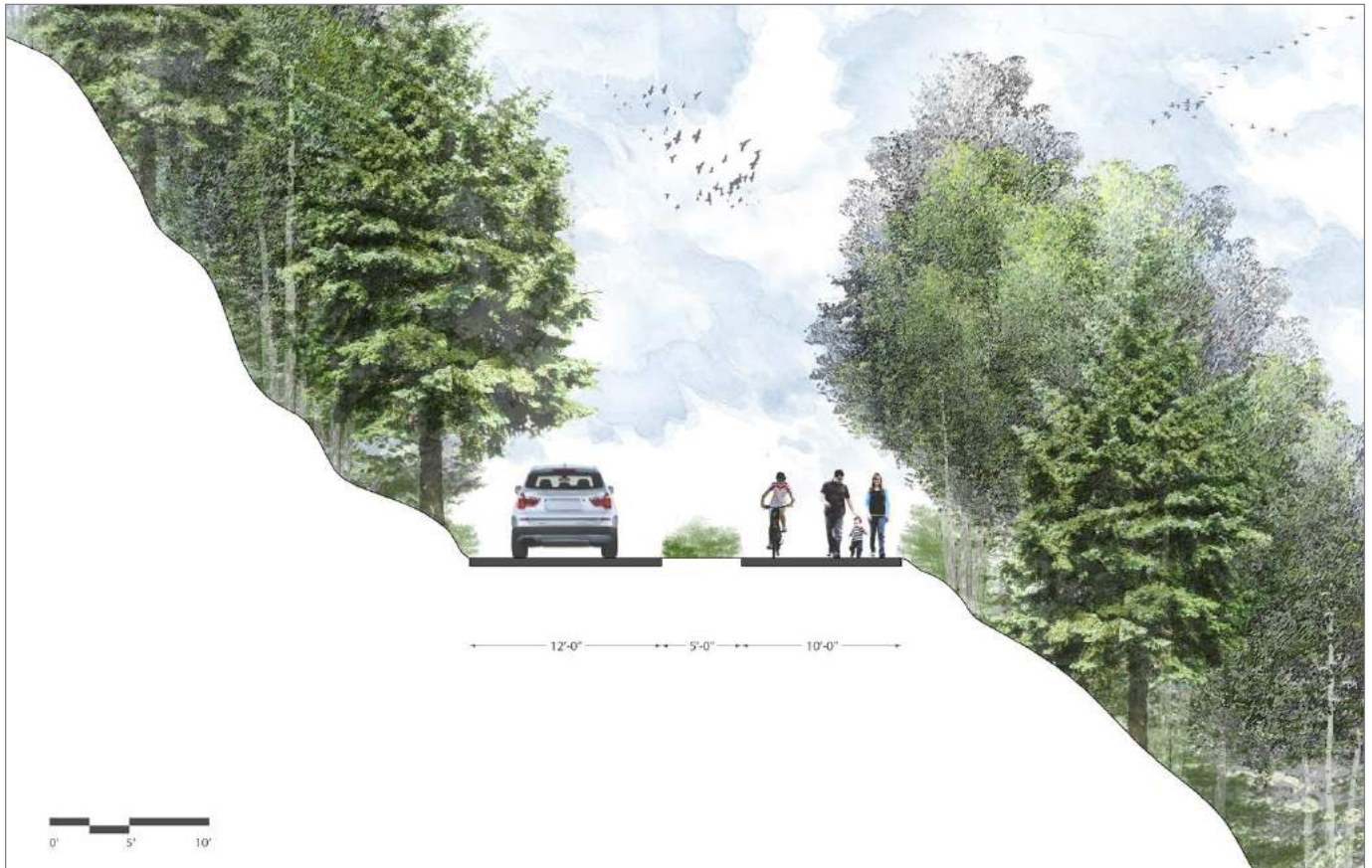
OPTION A: One-way vehicle traffic, vegetated buffer, and combined bicycle/pedestrian trail
