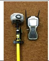
Fun Fact: GPS units are used for locating above and below ground infrastructure. Precision can be as high as 8mm horizontal and 15mm vertical. Respectively, that is within 1/3 and 2/3 of an inch.
