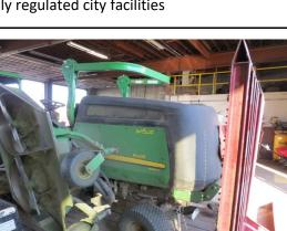
Fun Fact: This unit has 3 different mowing decks (2 side decks and a front deck) that can be operated
