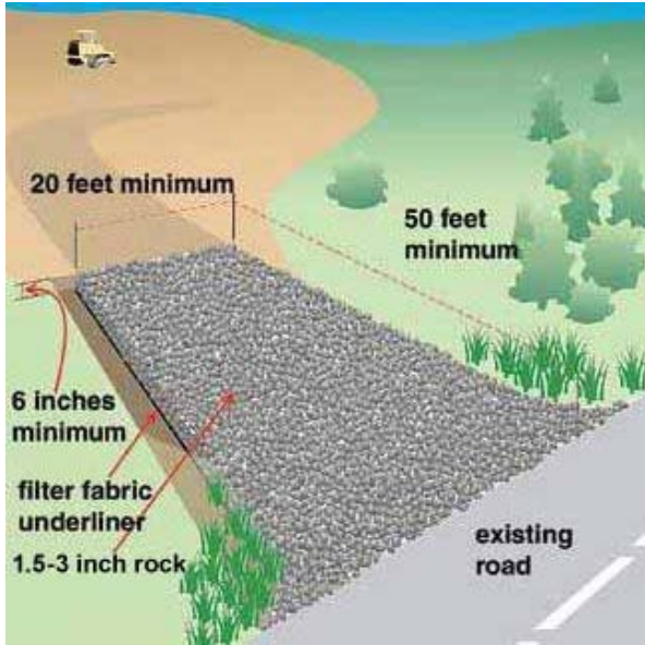
Rock Construction Entrance
